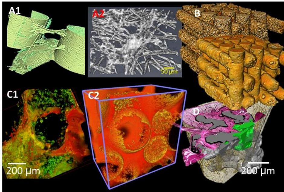
3D images of scaffolds with cells/tissues. A-Cells on 3D printed (A1) and electrospun (A2) scaffolds, B-sintering of bioactive glasses, C-protein adsorption (C1) and mineralisation (C2), D correlative imaging of bone-Ti-implants.
