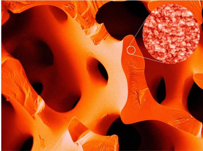
**Microstructure of a sea urchin spine (Scanning electron micrograph) – a biological mesocrystal. Although the spine has the properties of a single crystal, its morphology exhibits no crystal faces, which are typical for single crystals.**
